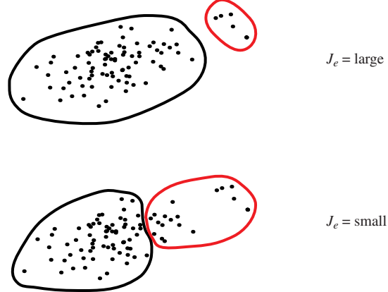
Figure 10.9: When two natural groupings have very different numbers of points, the clusters minimizing a sum-squared-error criterion (Eq. 49) may not reveal the true underlying structure. Here the criterion is smaller for the two clusters at the bottom than at the more natural clustering at the top.
